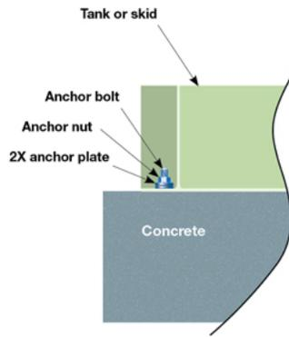
**Figure 5: Example of direct mounting to a foundation**
