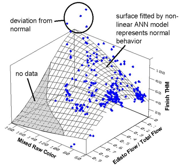
3D plot of ANN-based virtual sensor response surface fitted to measured THM data.
