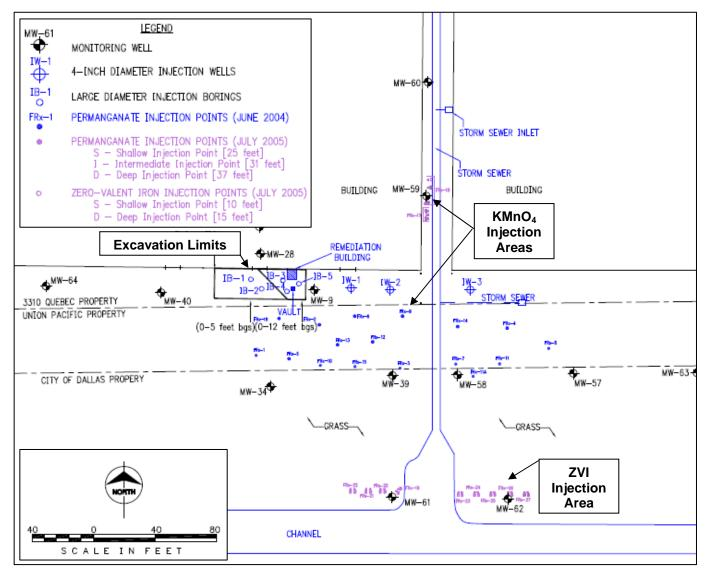
**Figure 1:** Areas targeted during June 2004 and June 2005 remedial activities – KmnO4 injected at caissons (IB-1 to IB-5) and fracture locations FRx-1 to FRx-18; ZVI injected at locations FRx-19 to FRx-27 along channel.
