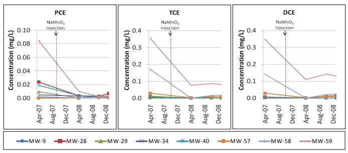
Figure 8: Effect of NaMnO4 injection conducted in October 2007.
