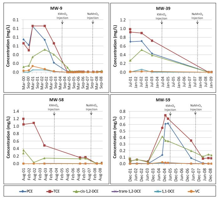
**Figure 7:** Effect of applications of KMnO<sub>4</sub> and NaMnO<sub>4</sub> at wells located at the source area (MW-9), directly downgradient from the source area (MW-39 and MW-58) and at isolated hot-zone (MW-59) targeted during the June 2004/2005 and October 2007 injection events.
