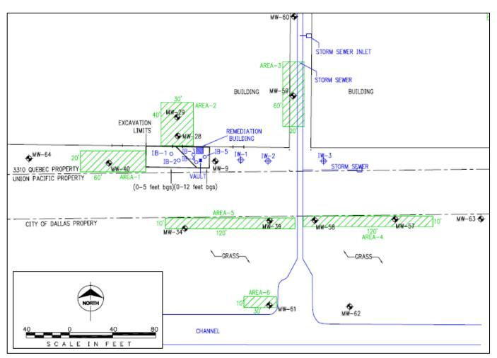
**Figure 2:** Injection areas October 2007 – NaMnO4 injected at Area-1 to Area-5 and EHC injected at Area-6.
