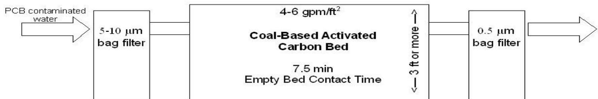
Overall, activated carbon adsorption is an effective way of reducing PCB contamination in groundwater. Successful results can be achieved with a properly designed system that addresses solids-control including both pre-filtration and post-filtration, along with proper carbon selection and bed design parameters including bed surface area, depth, and contact time.
