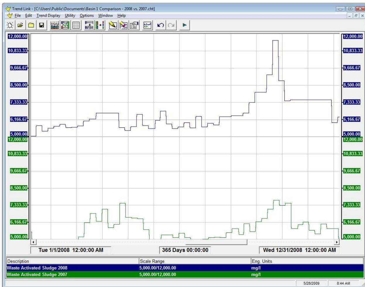
Figure 5: Being able to compare data from a previous run allows an engineer to spot what was different. Here, data from a run in 2008 is plotted against a similar run in 2007.
