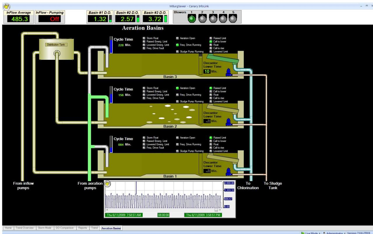
Figure 6: Canary InfoLink, a realtime and historical process analytic tool. A playback mode allows historical data to update the displays as if it was happening right now.
