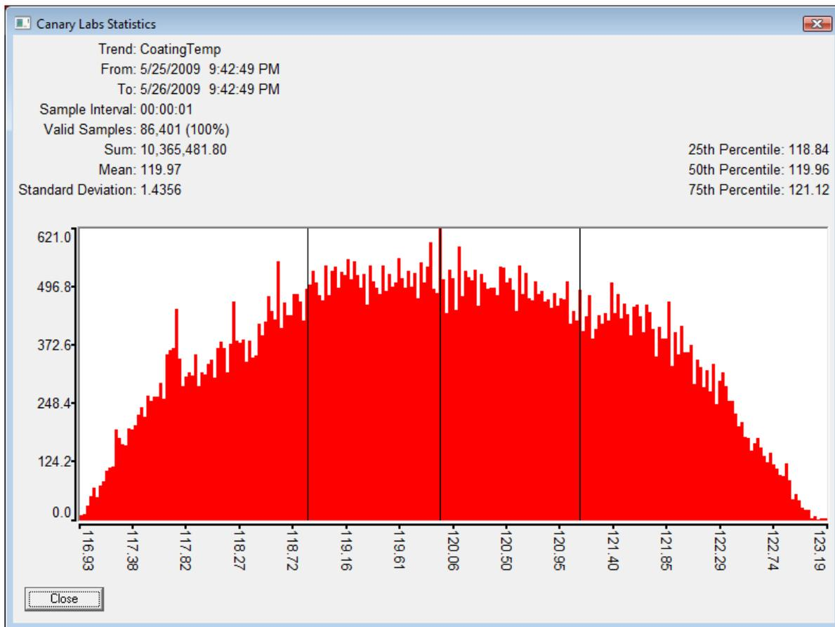
Figure 3: This histogram shows changes in coating temperatures over time. Note the statistical calculations for mean and standard deviation.
