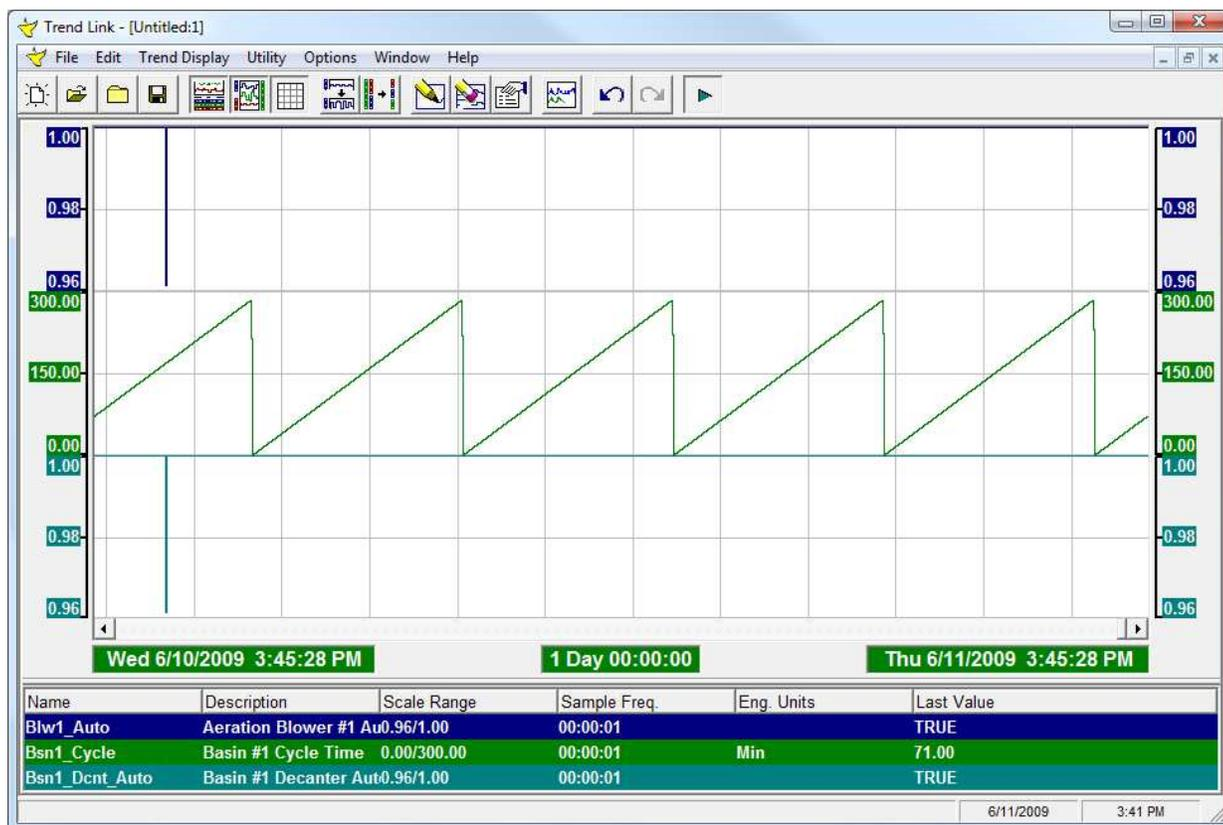
Figure 1: Real-time trend display which updates as new data is obtained.
