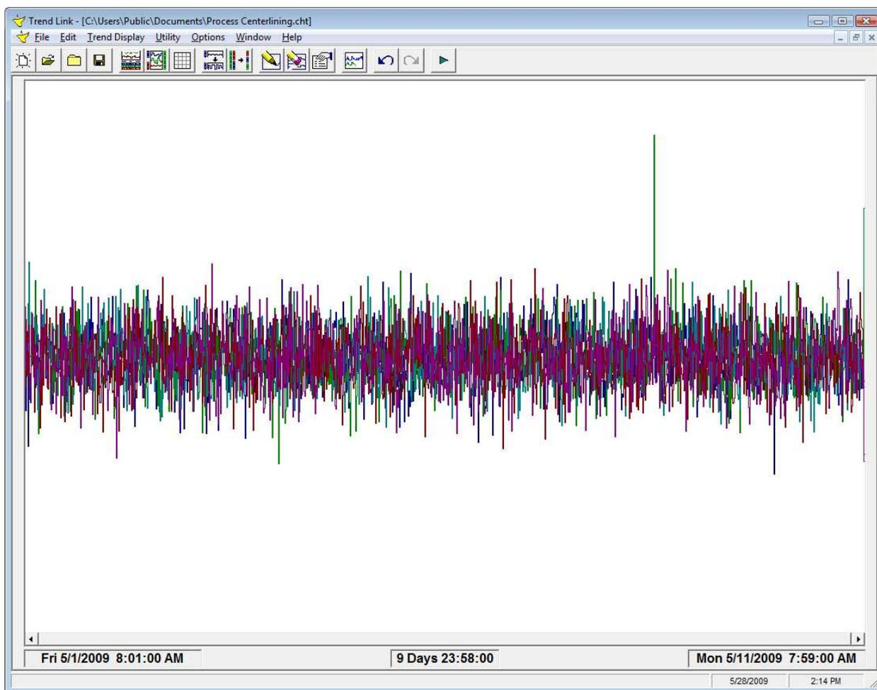
*Figure 2: Centerlining data—that is, arranging the plot so that multiple variables are centered on the screen—allows operators to spot “spikes” in the data and then drill down to examine the offending data in more detail.*
